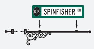
Loosen (4)  $10-24 \times 1/2$ " button head screws and dettach collar. Insert street blade into (2) channels, center and securelt tighten (2) 1/4-20 set screws.
