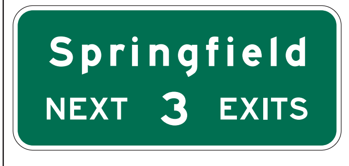
Figure 2E-33. NEXT EXITS Sign
