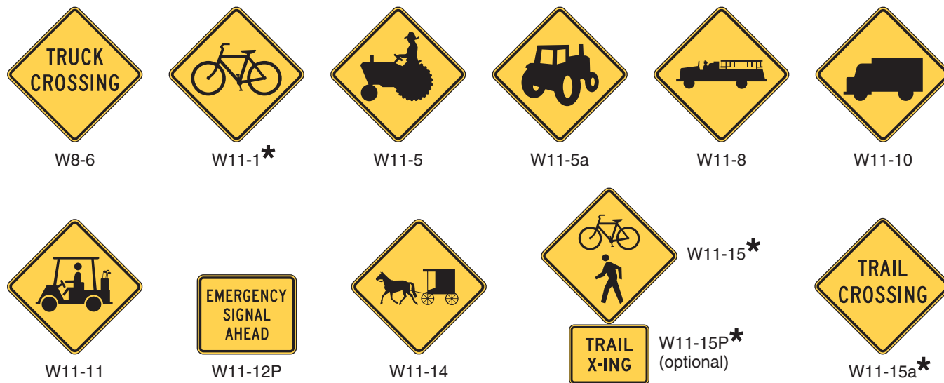
Figure 2C-10. Vehicular Traffic Warning Signs and Plaques
