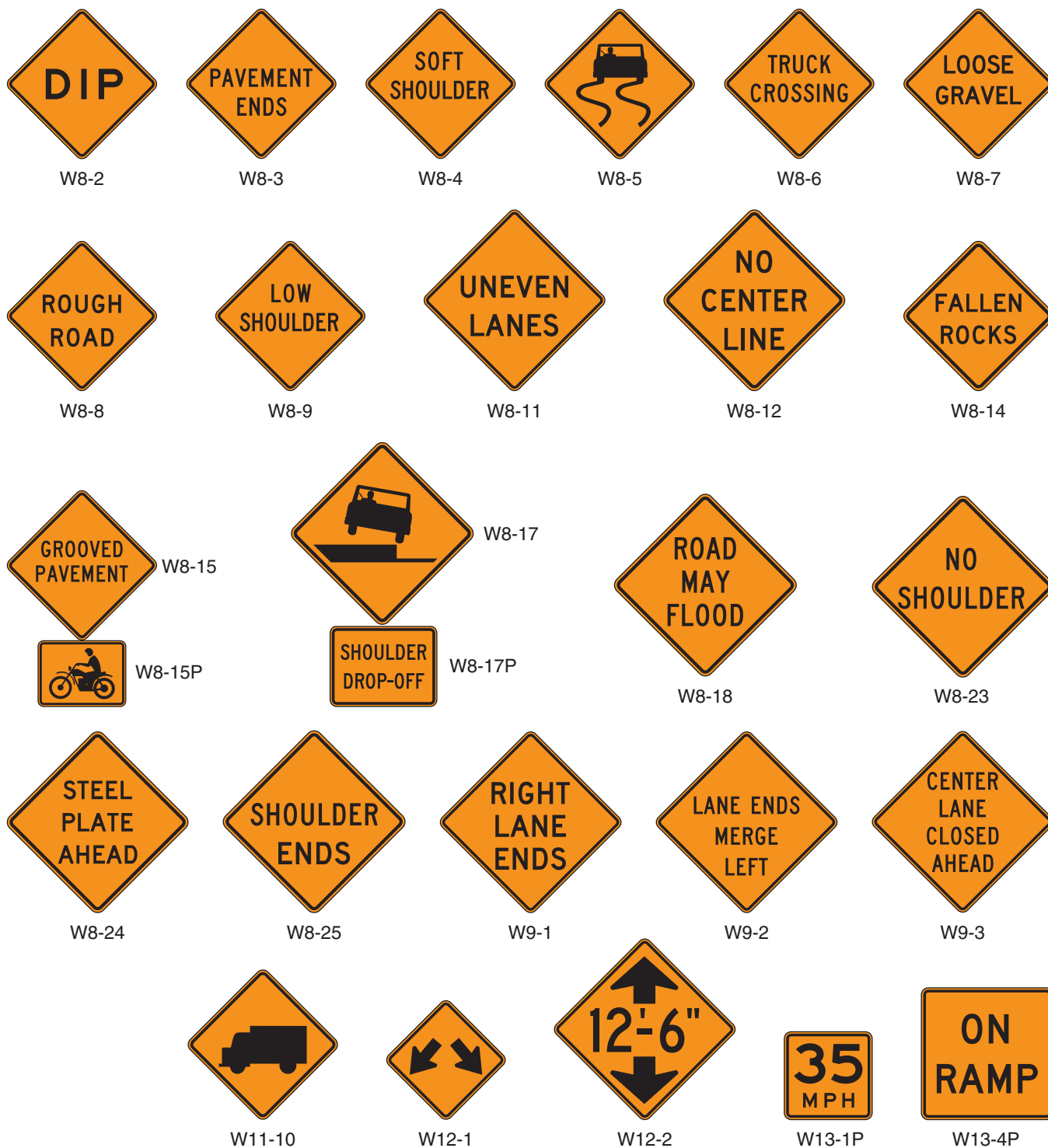
Figure 6F-4. Warning Signs and Plaques in Temporary Traffic Control Zones (Sheet 2 of 3)
