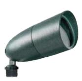
Low voltage MR16 flood with die cast aluminum housing, integral glare shield and tempered lens. Sleek good looks with minimal size. Supplied with 36" SPT-1 cord for installation on low voltage systems. MR16 lamp, 50 Watt max. Lamp not supplied.
