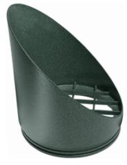
Die cast aluminum visor with integral metal grill and tempered glass lens for maximum glare reduction and lamp protection. Guard protects lamp from damage and vandalism. Die cast aluminum.
