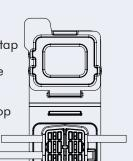
5. Using 8"-10" Straight Jaw, Groove Joint Pliers, individually press blade holders into housing until blade holder is fully seated in housing. Verify top surface of blade holder is even or just below the top surface of the housing.
