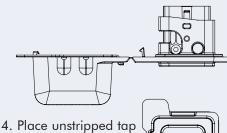
4. Flace Unstripped lap conductor into side B (see image in step 2). Insert conductor until visible against stop on opposite side.
