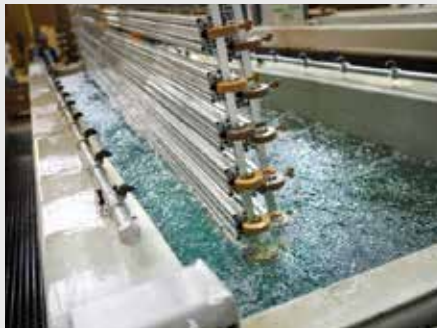
Bagno galvanico in polipropilene © Collini www.collini.eu
