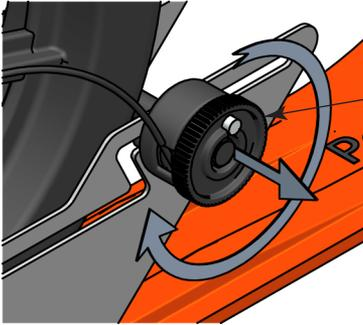
Place your wheels into the wheel cradles. Then pull the serrated part of the wire drum(1) out to unlock it. Hold the drum in the unlocked position and turn only the serrated part of the drum to feed out the wire.
