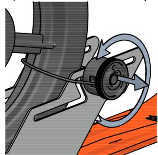
Wind in the slack on the wire leash(6) by pulling the drum out into the unlocked position then turn the drum to wind in the wire.
