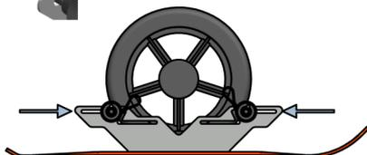
With the wheel fully seated in the wheel cradle(4) push the wheel pins(3) towards the wheel until they just touch the tire. Before you begin to tighten the hand nuts (2), make sure the pin is located into the slot.
