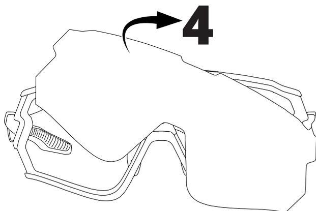
EN: To fit in a new lens repeat step 1-4 in reverse order (start with the insertion of the lens into the nose pad's handle).
