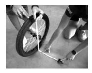
**5.** Using the correct allen wrench size, remove the rear wheel from your bike. If it is easier, you could remove the front wheel instead IF the tires are exactly the same size on the front and the back wheels.
