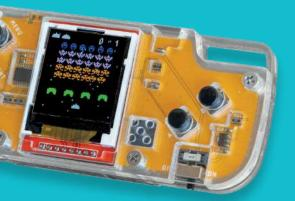
There are various types of displays. The one used on Nibble is called **the LCD display**.
