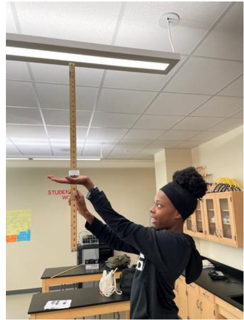
Exploring the relationship between distance and light intensity with databot™.
