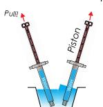
Tip: to work properly, no air bubbles should be in the cylinders or tubes.
