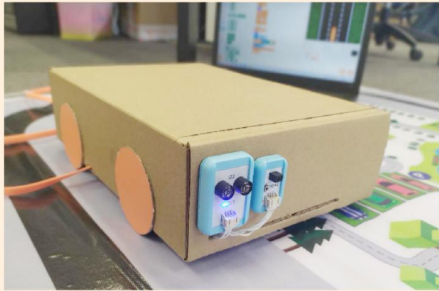
Rear side: Red LED is used to simulate the rear light of the car
