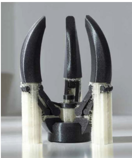
Dissolvable Materials like PVA and HIPS dissolve in water or specific solvent. HIPS requires constant high temperature of heated bed and environment.
