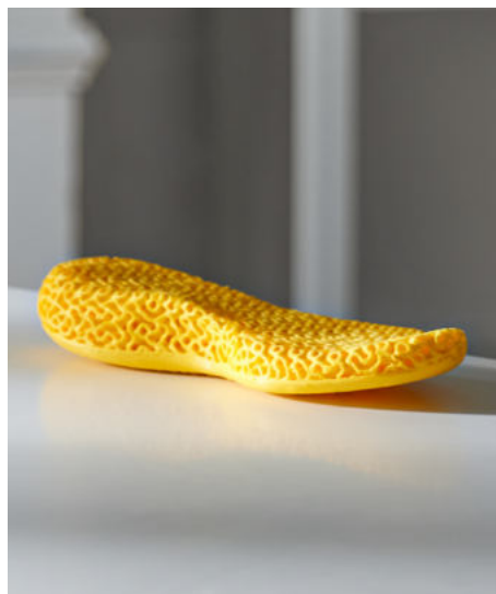
TPU Flexible and liable to over-extrusion and under-extrusion, and therefore requires accurate control of extrusion and heat dissipation.
