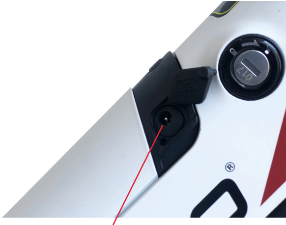
Slide open the protective hatch to access the charging port on the right side
