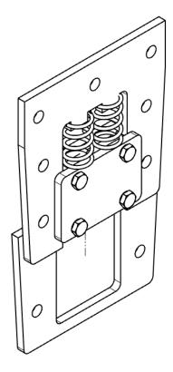
Place the spring on the locating lug of the W Iron and slide the axlebox into place. Then, slide the W Iron Keep in from the bottom. When the holes are aligned secure the keep in place with the M6 bolts and nuts.
