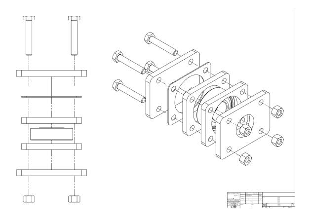
The axlebox is assembled in layers as shown in the diagram above. Use the M6 bolts and nuts to secure the plates together.
