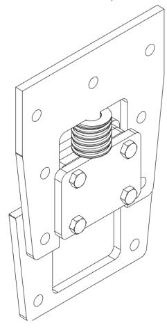
Place the spring on the locating lug of the W Iron and slide the axlebox into place. Then, slide the W Iron Keep in from the bottom. When the holes are aligned secure the keep in place with the M8 bolts and nuts.
