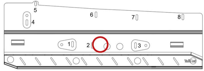
Distribute each Nylon spacer to the required position, using the Layout Guide for spacer allocations (pages 7 & 8)
