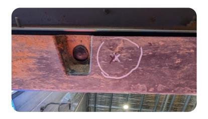
Using the 55-65mm Hole Saw bit, drill through the plastic below the bolt areas. Ensure the hole saw centre drill bit is just proud of the saw (<10mm) so you dont drill into the chassis.
