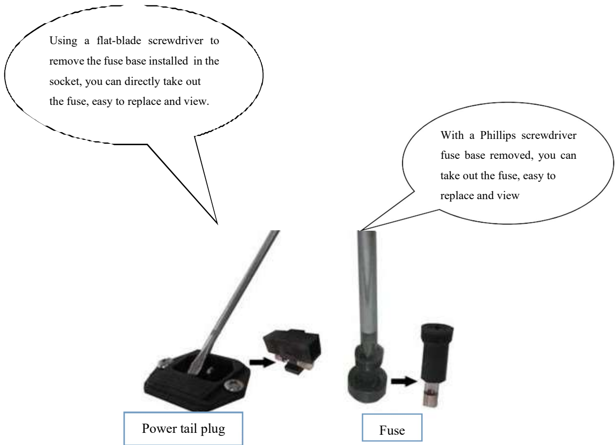
Figure 1 Fuse location and replacement
