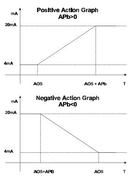
$\ensuremath{\mathsf{NOTE}}$  : When the defrost is in progress, the analogue output is set to the minimum value (4 mA). This condition lasts until the defrost terminates.
