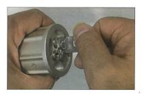
2. Using a mini flat head screwdriver, remove the counter part of the mini nozzle and wash with water. Screw back on the counter part into the mini nozzle, then screw the micro nozzle back into the main nozzle and tighten using the suggested nozzle tool.
