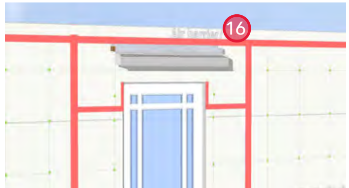
16. Install sheathing membrane from above and seal the leading edge with sheathing tape to maintain air barrier continuity. Ensure the sheathing membrane laps over membrane layers below.
