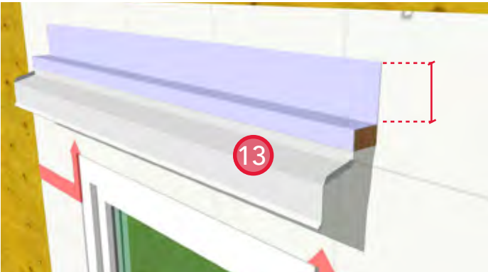
13. Install self-adhesive membrane over the prefinished metal flashing and extend 2" up the face of the wall.
