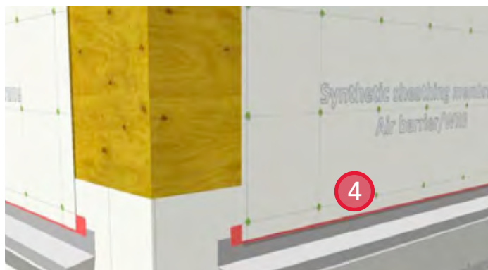
4. Install upper layer of sheathing membrane. Lap the membrane over the flashing.
