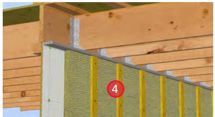
4. Install ROCKWOOL COMFORTBOARD™ 80 and strapping with bugscreens, leaving a 3/4" gap to ensure air barrier continuity through sheathing to rim joist interface. Suggest using a 1x4 temporary spacer board to space the insulation.
