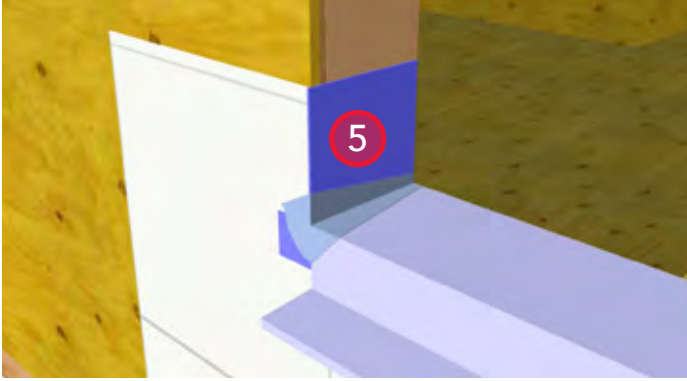
5. Install self-adhered membrane gussets at lower corners.
