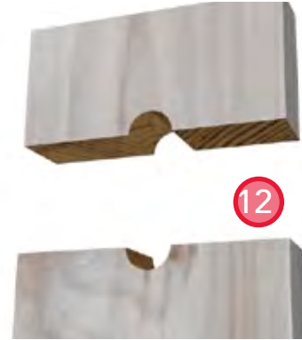
12. Create the wood face plate from dimensional lumber. The diameter of the hole in the center is equal to the diameter of pipe on the hose bib.
