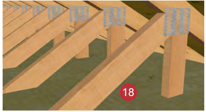
18. Install ROCKWOOL COMFORTBATT® in the attic to the depth necessary to achieve desired R-value.
