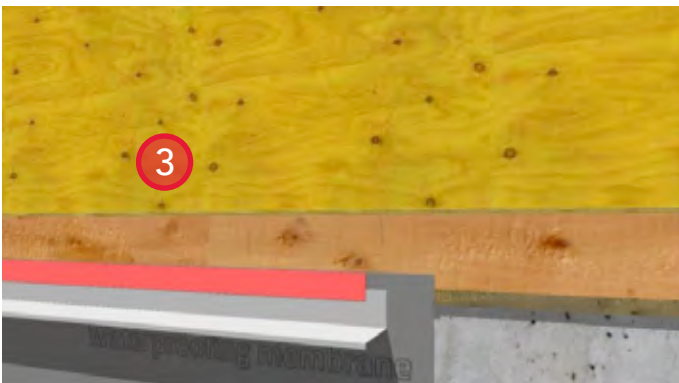
3. Install prefinished metal flashing and seal leading edge to the underlying waterproofing membrane with sheathing tape to provide for air barrier continuity.
