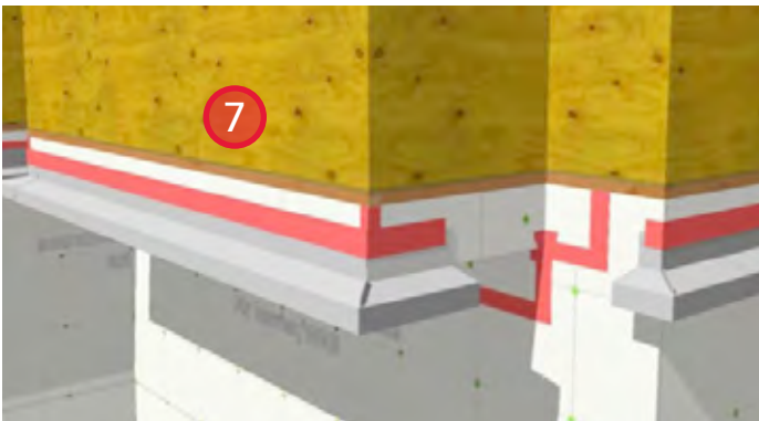
7. Seal the leading edge of the flashing backleg with sheathing tape to provide for air barrier continuity.
