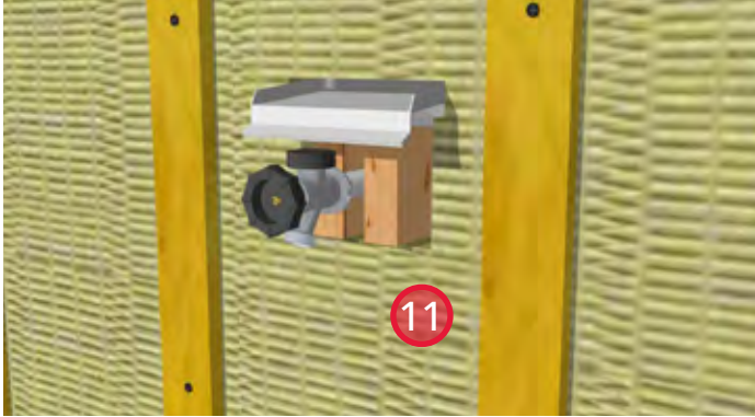
11. Install ROCKWOOL COMFORTBOARD™ 80 and strapping. Provide bugscreens at the top and bottom of the strapping.
