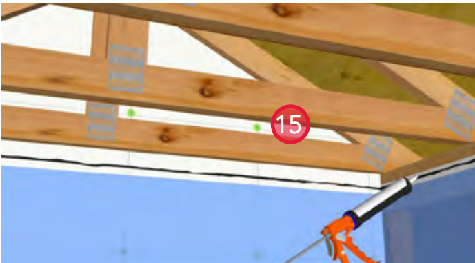
15. Install a bead of acoustical sealant along the sheathing membrane in line with the lower top plate of the exterior wall.
