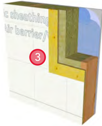
3. Install sheathing membrane.
