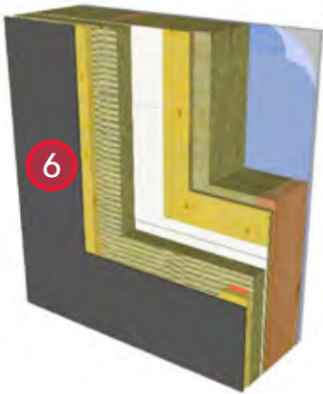
6. Install backer board.
