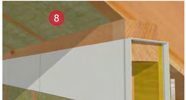
8. Install ROCKWOOL COMFORTBATT® in the stud cavities and roof cavity. Provide venting per building code requirements.
