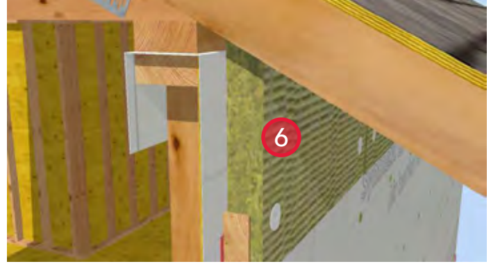
6. Install ROCKWOOL COMFORTBOARD™ 80 and secure with recommended fasteners.
