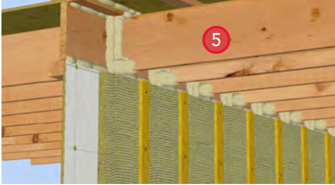
5. Remove the spacer board and install 2 lb. closed-cell spray foam or sealant at all joints in the joist cavity to maintain air barrier continuity.
