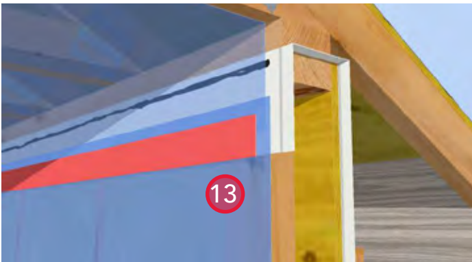
13. Install poly to the underside of the roof rafters and fasten with staples at the sealant bead to complete the air seal. Seal the leading edge of the poly with sheathing tape to maintain vapour barrier continuity.
