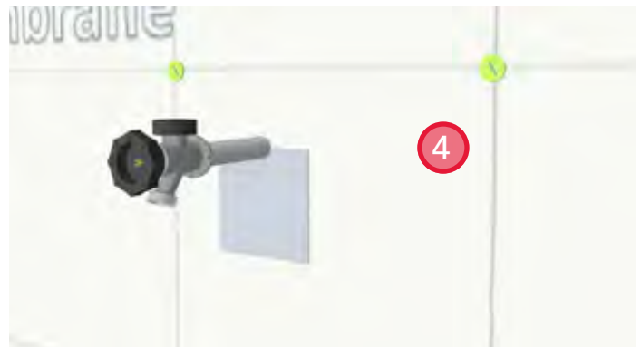
4. Install the bottom sheet of foil-faced, self-adhered membrane, ensuring a tight fit to the underside of the hose bib.
