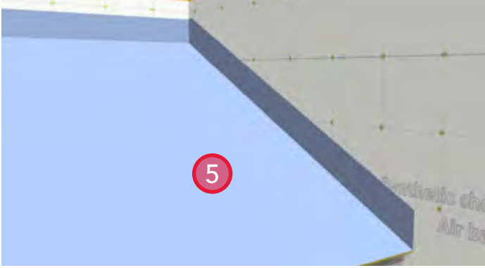
5. Install waterproof roof membrane. Return the membrane up the vertical face of the adjoining walls 1" beyond the projected back leg of the closure flashing.
