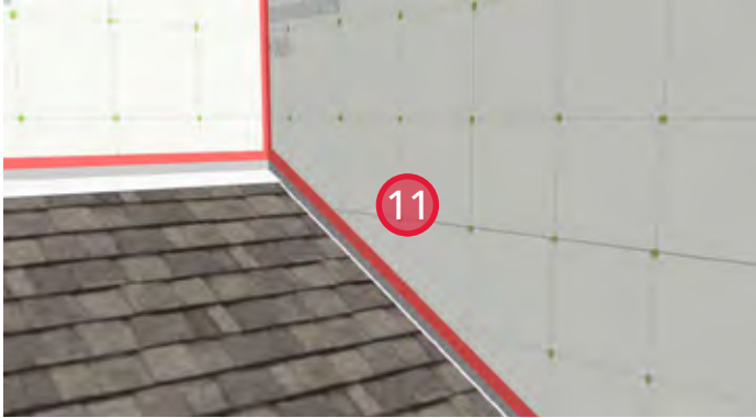
11. Seal all edges of the sheathing membrane with sheathing tape.
