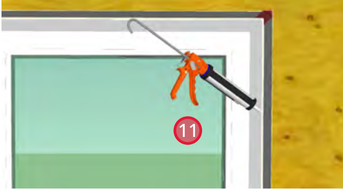
11. Install backer rod and sealant around the interior perimeter of the window to complete air barrier continuity.
