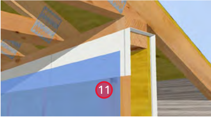
11. Install poly and fasten to the sheathing membrane at each stud with staples.
