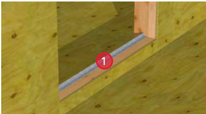
1. Typical wood frame rough opening for swing door. A back angle has been installed in the rough opening to aid in water diversion.
