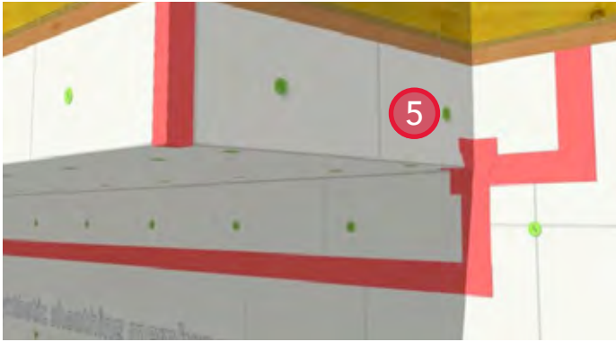
5. Install gussets constructed of sheathing tape to cover the pinholes at the inside corners.
