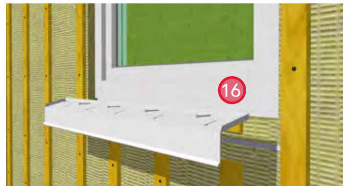
16. Install prefinished metal sill flashing. Attach the sill flashing to the nailing flange under the window sill.
