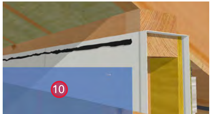
10. Install a bead of acoustical sealant on the sheathing membrane at the lower top plate to transition the air barrier from the wall to the ceiling.
