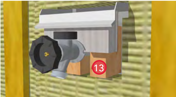
13. Install the top piece of the wood face plate and secure in place.
