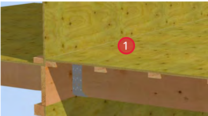
1. Typical wood frame construction at joist hanger supported balcony to above grade wall interface.
