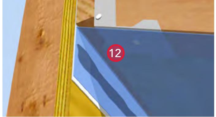
12. Install poly and seal the leading edge to the sheathing membrane with staples through the poly at the sealant bead to complete the air barrier transition.
