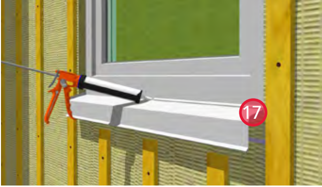
17. Apply sealant between the metal flashing and the window sill.
