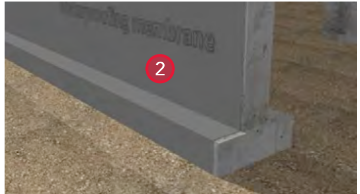
2. Install the below-grade waterproofing membrane. Ensure the membrane wraps over the footing and terminates on the vertical.
