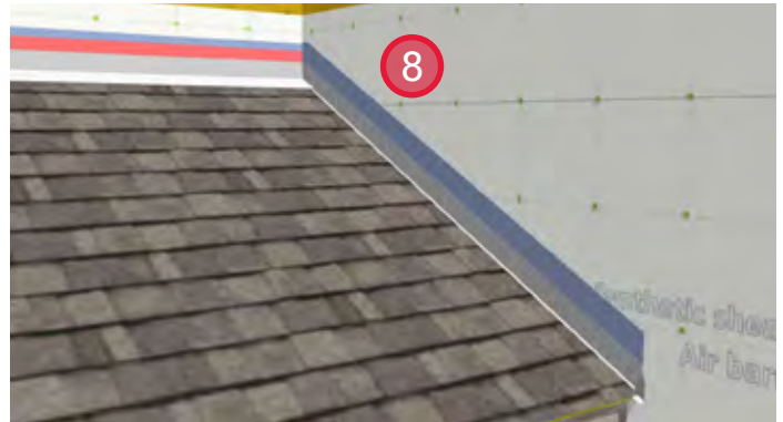
8. Install prefinished metal closure flashing on the above wall and seal the leading edge with sheathing tape.
