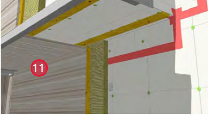
11. Install cladding and vented soffit material.
