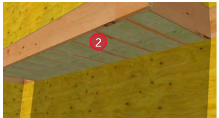
2. Install ROCKWOOL COMFORTBATT® in the cantilevered floor joist cavities. Ensure insulation extends through to the interior plane of the wall assembly to maintain thermal continuity.
