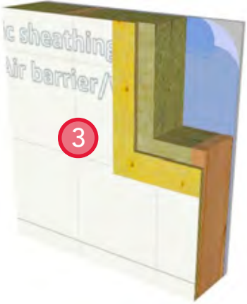
3. Install sheathing membrane.
