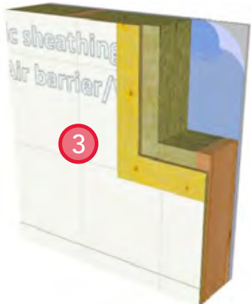
3. Install sheathing membrane.
