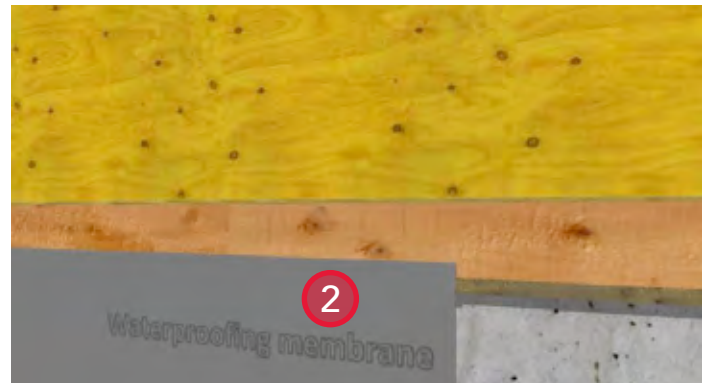
2. Install below-grade waterproofing membrane. Provide a 2" overlap of waterproofing membrane onto the sheathing.
