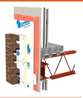
SOPRASEAL STICK 1100 T is a self-adhesive air/vapour barrier membrane for walls composed of SBS modified bitumen and a tri-laminate woven polyethylene facer. It is also used as masonry and through-wall flashing membrane as well as waterproofing membrane at openings and transitions.
