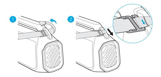
• Attach the strap to both sides of the handle.
