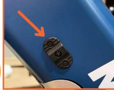
Lastly, push the battery latch on the opposite side of the downtube downwards toward the pedals. The battery is now secure and you can remove the keys.
