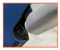
Place the end of the battery into the lower part of the cradle so the battery connections line up.
