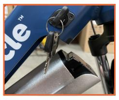
You can now gently pull the battery down and forward towards the handlebars to release the battery completely.
