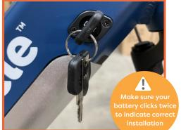
Push in again and you should hear a second click. This second click indicates your battery is now securely locked in place. The key will also turn fully to the lock position by itself.
