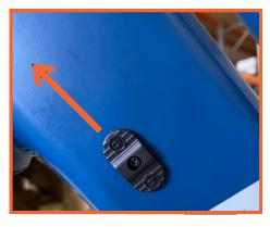
On the opposite side of the bike, is your battery latch. Slide this upward toward the bars to the unlock position.
