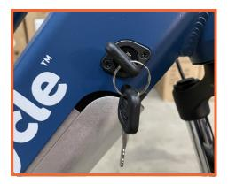
Place your hand under the battery. Go back to your key and turn it counter clockwise to the unlock position. The battery should pop open with this action to indicate it has unlocked.
