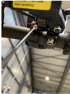
2-Then using a 3mm hex key undo the bolt underneath the display unit.
