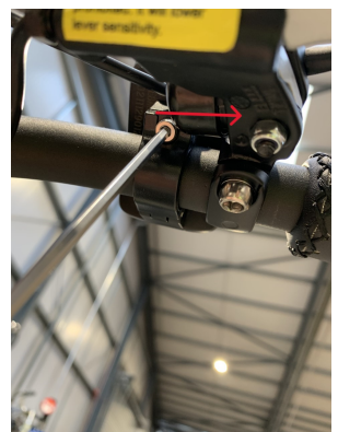
6-Then using a 3mm hex key attach the bolt underneath the display unit.
