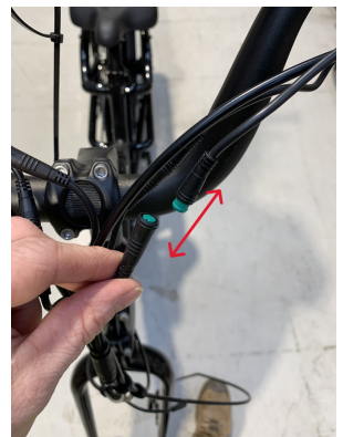
3-Follow the cable out of the display unit to the connection bellow, unplug it.
