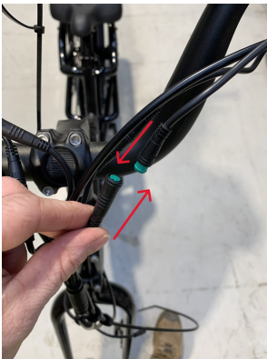
4-Plug in your new display unit to the cable you have just unplugged your old one from. When plugging in the new cable be sure to follow the pin configuration.
