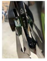
6. To remove the pads simply squeeze the pads together into the center of the opening with your fingers or pilers and pull out.
