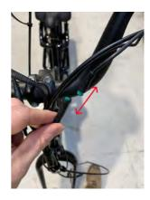
3-Follow the cable out of the display unit to the connection bellow, unplug it.
