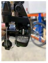
9. You are now ready to replace or refit your brake pads. Use a flat headed screwdriver to push the pistons back into the caliper body. Place the pads back into the caliper body with the return spring clipped over the braking surface of the pad. Line up the eyelet hole with those on the caliper body. Refit the split pin and bend the longer edge out to secure it.
