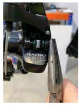
5. Using the pliers straighten out the bent end of the split pin and pull through. This will release the pads and return spring. The pads will be loss to be sure they do not fall out.
