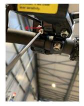
2-Then using a 3mm hex key undo the bolt underneath the display unit.
