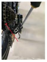
3- Using the limit screws 'H' screw using a Philip's screwdriver turn counter or clockwise to align the derailleur to sit directly above the small sprocket (indicated).
