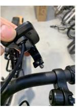
5- Place the new display unit on handle bar.
