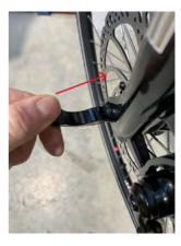
10. Fit your wheel back in being careful to line up the disc to sit in-between the pads. Now tighten the wheel nuts or quick release back up.
