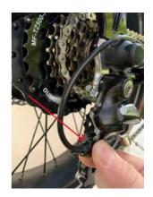
8- If you find a gear that the derailleur is struggling to shift up into. Using the barrel adjuster located at the point the gear cable joins the derailleur. Turn this counterclockwise one click at a time till the chain changes into the selected gear.
