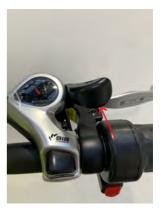
4- Using the trigger on the top side of the shifter click through until it stops.
