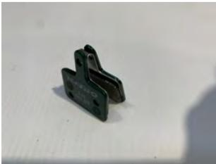
8. When inspecting your brake pads look for any damage to the pad surface and any discoloration. The pad should have clear dark or light grey metallic appearance. If there is any discoloration on the pad you should only use a bicycle disc brake cleaner (ensure you follow the instruction on the can) and a clean rag to clean the pad.
