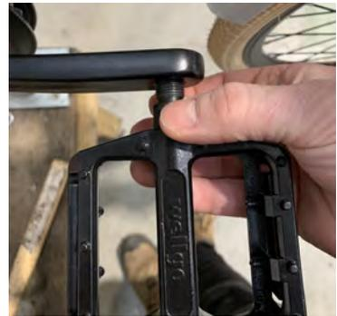
There should not be any resistance as you tighten. If you are experiencing resistance stop and undo the pedal, inspect the thread for damage and start again.
