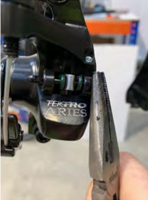
5. Using the pliers straighten out the bent end of the split pin and pull through. This will release the pads and return spring. The pads will be lost to be sure they do not fall out.
