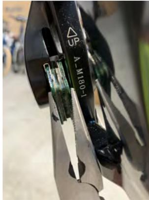
6. To remove the pads simply squeeze the pads together into the center of the opening with your fingers or pliers and pull out.
