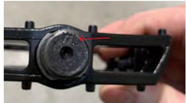
Once you can see and are sure the pedal has entered the crank straight you can now use a 15mm spanner to tighten the pedal till you can no longer see the thread.
