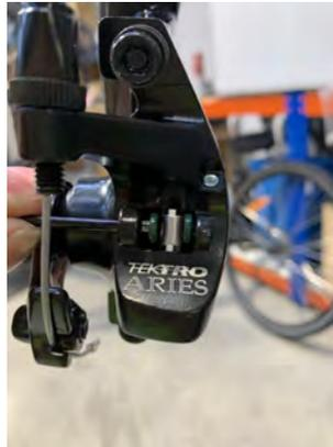
9. You are now ready to replace or refit your brake pads. Use a flat headed screwdriver to push the pistons back into the caliper body. Place the pads back into the caliper body with the return spring clipped over the braking surface of the pad. Line up the eyelet hole with those on the caliper body. Refit the split pin and bend the longer edge out to secure it.
