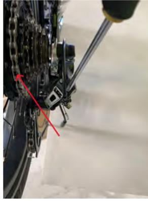
3- Using the limit screws 'H' screw using a Philip's screwdriver turn counter or clockwise to align the derailleur to sit directly above the small sprocket (indicated).
