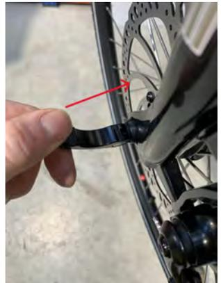
10. Fit your wheel back in being careful to line up the disc to sit in-between the pads. Now tighten the wheel nuts or quick release back up.
