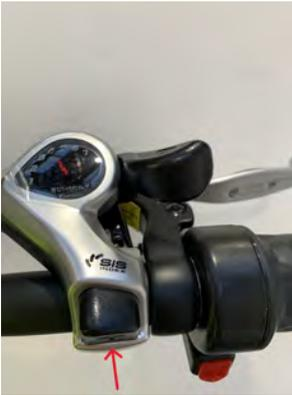
2- Using the gear shifter press the trigger that sits in line with the handle bar. Click through all the gears till it stops clicking.
