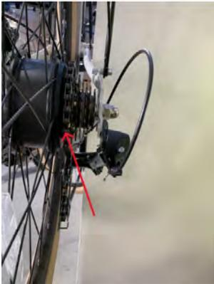
5- Using a Philip's screwdriver this time on the 'L' screw, turn counter or clockwise till the derailleur sits directly above the largest sprocket.
