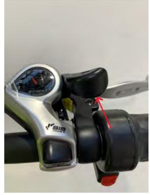
4- Using the trigger on the top side of the shifter click through until it stops.
