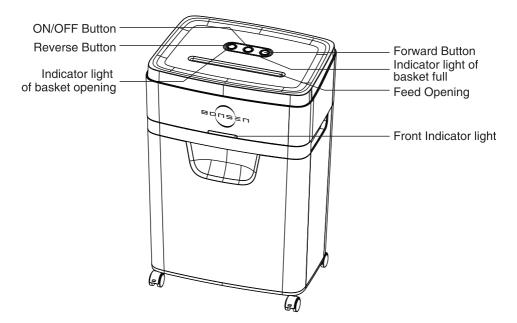
**REV Button:** To make the paper rise up when the shredder gets the trouble in paper jam.
