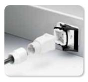
Thanks to insulation displacement connection, it now only takes a few seconds to connect the 4-pole round conductor: Only the sleeve nut has to be slid over the conductor – since splicing ring, seal and strain relief are included in the sleeve nut.
