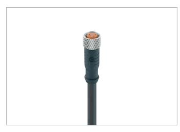
M8 actuator/sensor cordset with overmolded connector, with self-locking threaded joint, IP 67 Cable end 1: M8 female connector, straight, A-coded Cable end 2: blunt cut Cable: PUR, black
