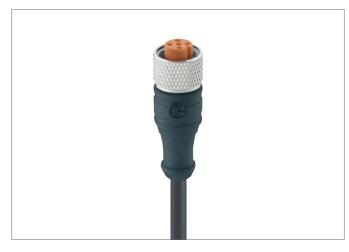
M12 actuator/sensor cordset with overmolded connector, with self-locking threaded joint, IP 67 Cable end 1: M12 female connector, straight, A-coded Cable end 2: blunt cut Cable: PUR, black
