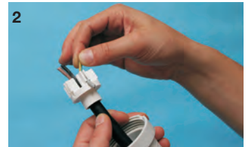
Then lead all five conductors through the distributor ring. Draw one after the other conductor sideways into the marked connection chambers. No stripping required.
