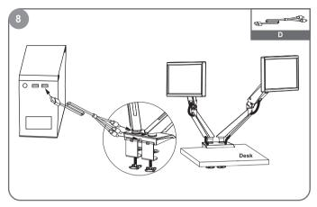
Connect USB plug of supplied cable to USB port on your desktop computer or laptop. LED lighting on monitor mount will illuminate once connected.
