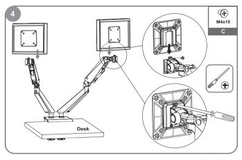
Insert the monitor along with the VESA plate to the arm with screw (M4x10) using screwdriver and lock it.
