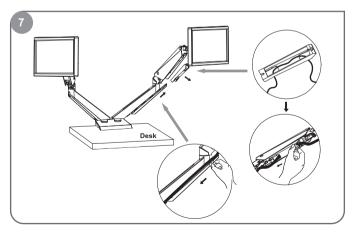
Remove the cable cover from extension arm. Feed the cables along the arms and replace the cable cover.
