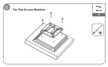
Flush surface installation: Install 4 screws (M4x12) through faceplate to monitor via mounting the holes.
