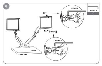
Use 5mm Allen Key to adjust the arms for swiveling and tilt movements. Turn counter-clockwise to reduce movement and clockwise to increase movement.
