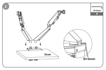
Install the arm to the base. Fasten the screw in the back with 3mm Allen Key.
