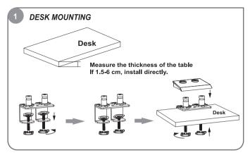
Loosen clamp screw until enough space is left for the edge of the desk. Tighten clamp using clamp screw until mount is securely fastened to desk.
