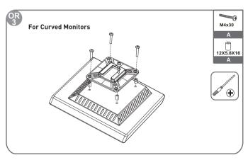
Recessed surface installation: Put 4 spacers (12x5.8x16) between faceplate and monitor. Use screwdriver to install 4 screws (M4x30) through faceplate and spacers to monitor via the mounting holes.
