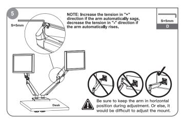
Use 5mm Allen Key to adjust the height tension of the gas spring arm, to keep different weight of monitors still at any position.
