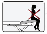
Do not sit or put unnecessary amounts of pressure on the back section of the table when it is in tilt position of any level. This can damage or destroy the tilt mechanism and cause harm or bodily injury to persons. The tilt mechanism is intended solely to be used when a client is properly seated or laying on the table top. Damage caused in this manner may void the warranty.
