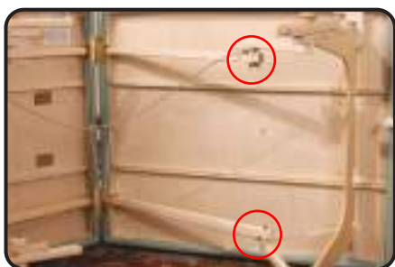
6. Remove the Shiatsu cables or bolts on one side to enable your table to lay flat. There are different types of shiatsu cables. Follow these directions based on the type you have. Or follow your table manufacturer's instructions.
