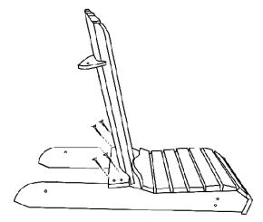
Step 2, fit the back to the seat and align edges. Fasten 4 screws.
