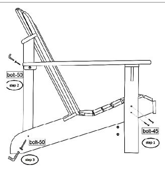
Step 4, Attach front legs to side legs with 4 bolt-45 and nuts. Attach the rear of armrest to rear leg with 2 bolt-50 and nuts.
