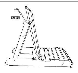
Step 3, attach 2 rear legs to the back with 2 bolt-35 by allen key.
