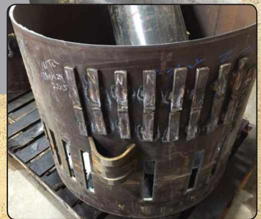
An excellent tool for making coupons for bend, tensile strength, and hardness tests.
