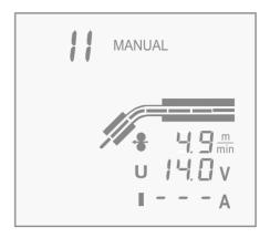
In Manual mode you can select from two different arc dynamics settings. Press Manual mode button (Arc Dynamics control on MinarcMig 170 model) once to pre-select either arc dynamic value I or value II. Changing between setting I and setting II will adjust the short circuit characteristics to suit different welding applications.
