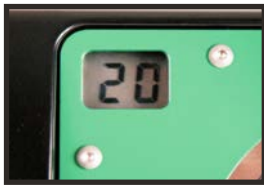
The grinding angle is shown in the digital readout.
