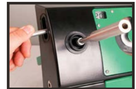
TIP-TRIMMER is able to cut and grind electrodes as short as 10mm in length.
