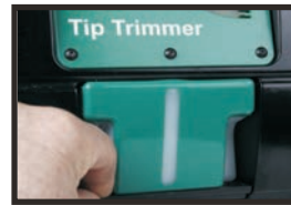
The waste container is easy removed from the front.
