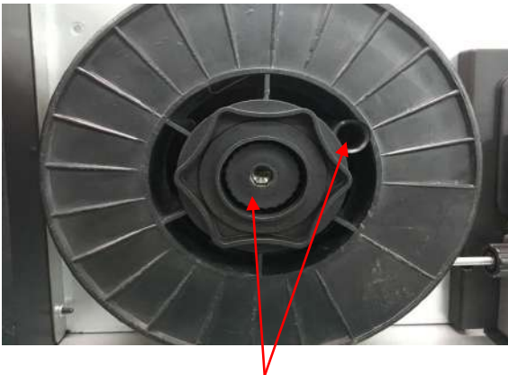
(3) Fit the wire spool onto the spool holder fitting the locating pin into the location hole on the spool. Replace the spool retaining nut tightly.
