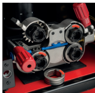
Compact 4-roller quick-release wire feed unit with insertion rollers ( \varnothing 37 mm), easily identifiable thanks to color-coding system through diameters
