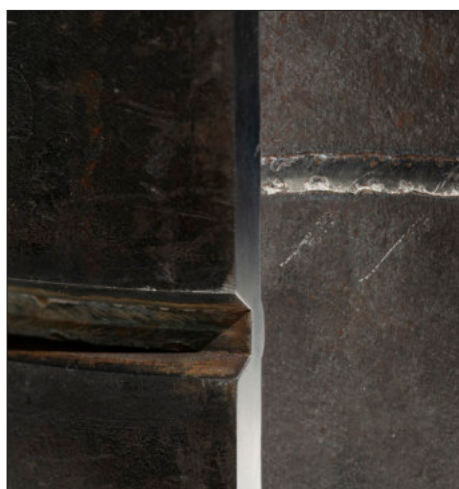
MIG SRS - First pass on tube with beveling
