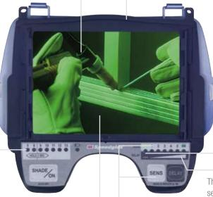
The "tack welding comfort mode" uses an intermediate light state (shade 5). If a follow-up arc is not struck within two seconds, the welding lens switches to the normal light state (shade 3). The comfort mode helps reduce eye fatigue resulting from the eye constantly needing to adjust to differing light levels during tack welding.
