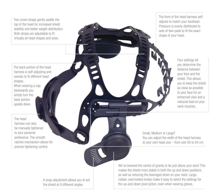
Welders who keep their shield in the down position for prolonged periods of time complain of discomfort from stale air and reduced vision from humidity fogging up the lens inside the shield.
