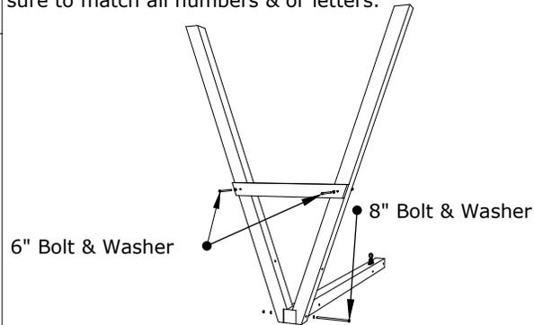
3. Attach 2 (C) Top Braces to (A) Beam & (B) Legs using 2 - 5/16 x 6" Bolts 4 Washers & 2 - 5/16" Nuts for Legs. Install 1 - 3/8" x 9" Bolt 2 Washers & 1 - 3/8" Nut for Beam. Be sure to match all numbers & or letters.
