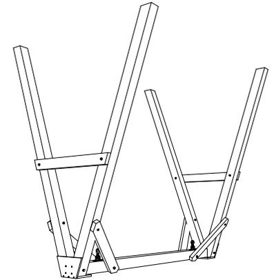
5. Attach (E) End Caps using 8 - 2" Screws per End Cap in predrilled holes. Be sure to match all numbers & or letters.
