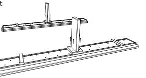
Attach (B) Top to (D) Legs Using 8 - 2-1/2" Stainless Screws in Predrilled Holes.
