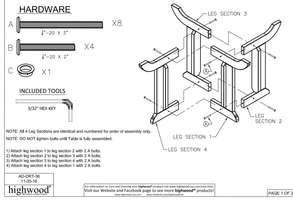
DO NOT fully tighten the bolts until all bolts are started. Once all bolts are inserted, then go back and tighten all the bolts.
