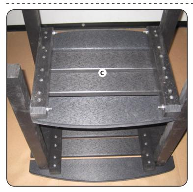
**Step 2**Attach one of the shelves as shown (C), with (4) 1/4" x 3 1/2" bolts and (4) 1/4" flange nuts, one per leg. Repeat with the other shelf (not shown).
