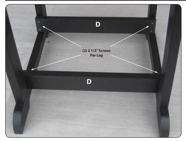
Step 3 Set the table upright and fasten the table support braces(D) on the inside of legs with (2) 2 1/2" screws per leg.
