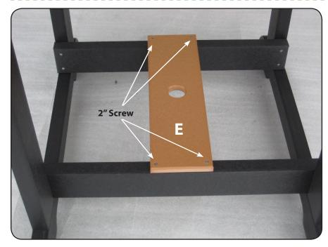
**Step 4** Place the umbrella support brace onto the table support braces. Measure carefully to align it with the umbrella hole on the table top. Fasten with (4) 2" screws, 2 on each side.
