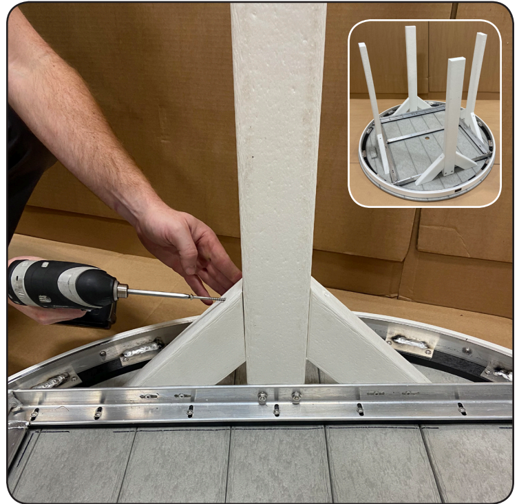
Step 5 On the other side of the leg, attach another brace in the same manner as Step 3 & Step 4. Repeat with three remaining legs and six remaining braces.
