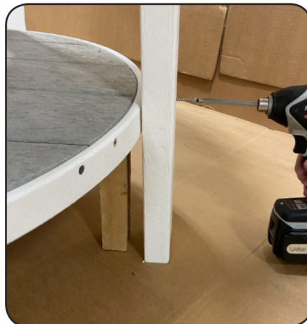
Step 5 Stand the table upright, and place the (2) stilts (E) in place as pictured left. Set the shelf (D) onto the two stilts to hold it up during installation, making sure the shelf is turned the same way as the table top above, so the boards run parallel with each other, then fasten the shelf to the legs through the holes provided with (8) 2 1/2" screws, 2 per leg. Discard stilts.
