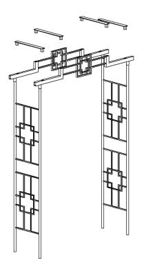
STEP THREE: WITH A LADDER, SLIDE IN THE FOUR TOP ACCENT PIECES INTO THE TWO TOP SECTIONS.
